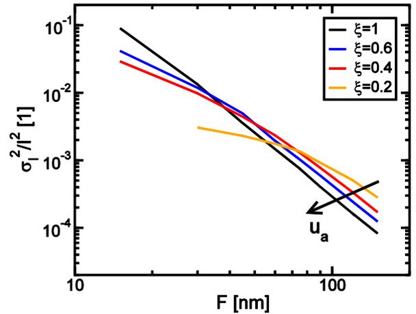
**Fig. 6** Calculated average  $\Delta R/R$  as a function of  $F$  for various aspect ratios  $\xi = u_a/\sqrt{A}$  of the amorphous volume. Isotropic scaling approach was assumed in the calculations [12].
