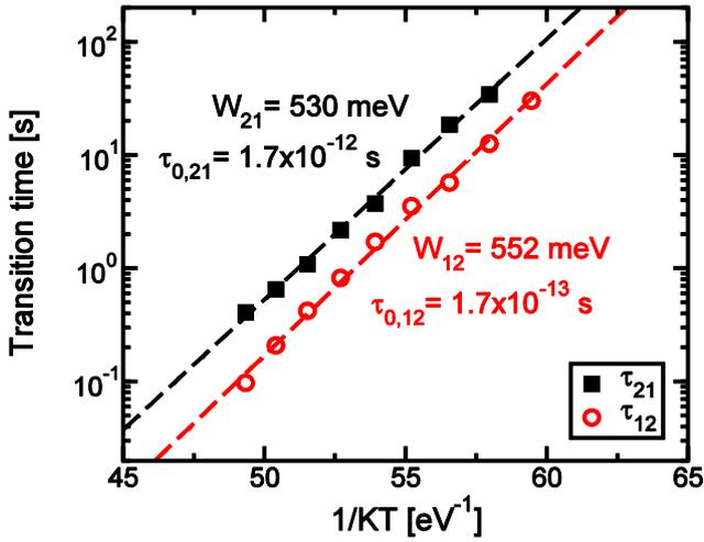
**Fig. 3** Measured transition times  $\tau_{12}$  and  $\tau_{21}$  in the Arrhenius plot. Times were obtained from the time-domain analysis of data in Fig. 1. Arrhenius fitting from Eq. (4) is also shown [12].
