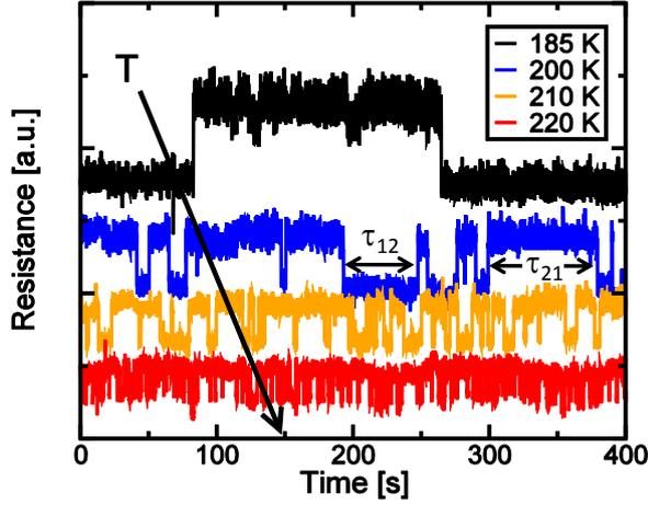
**Fig. 1** Measured  $R$  as a function of time for increasing  $T$ . The measured resistance clearly displays RTN with increasing amplitude and transition times for decreasing  $T$  [12].
