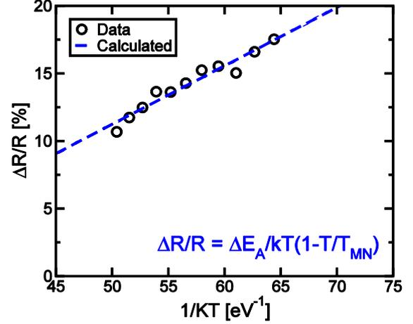
**Fig. 2** Measured  $\Delta R/R$  from Fig. 1, as a function of  $1/kT$ . The linear behavior indicates a change of activation energy for conduction  $E_A$  as the root cause for the two-level conductance fluctuation [12].
