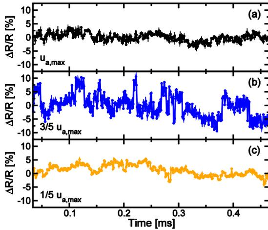
**Fig. 5** Calculated  $R$  as a function of time for amorphous thickness  $u_a = u_{a,max}$  (a),  $3/5 u_{a,max}$  (b) and  $1/5 u_{a,max}$  (c) [12].
