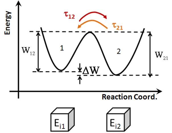
**Fig. 4** Schematic energy diagram for bistable fluctuation at the basis of RTN. The small  $\Delta W$  leads to slightly different transition rates between the metastable states [12].
