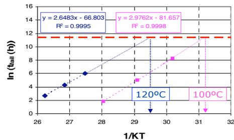
**Fig.5** Evaluation of activation energy for crystallization, based on analytic cell (blue) and macrocell (pink) data.
