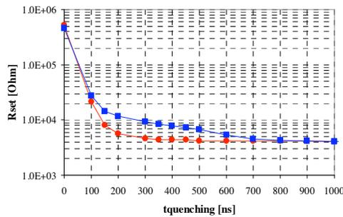
**Fig.2** Set level as function of trailing pulse length on analytic cell. Degradation in Set performances is due to not optimized heater-precontact interface (blue curve).
