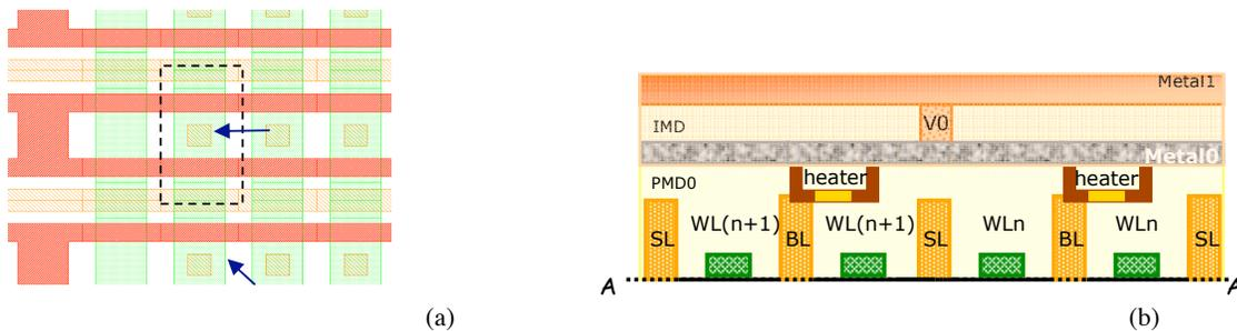
**Fig.1** Schematic layout of the MOS-selected PCM cell (a) and cross section along Bit Line direction (b). Two transistors in parallel address the same storage element and common source is biased by local interconnect.
