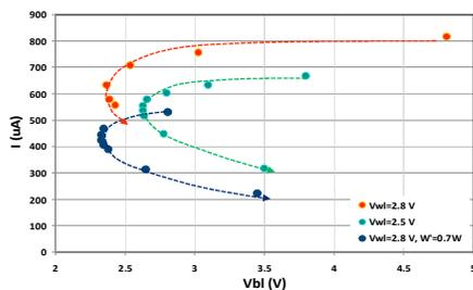
**Fig.3** Cell working point optimization (TCAD results). Expected programming current as function of Bit Line voltage is reported at different Word Line voltage (2.5-2.8V) by varying heater resistivity. Constant dissipated power is considered.
