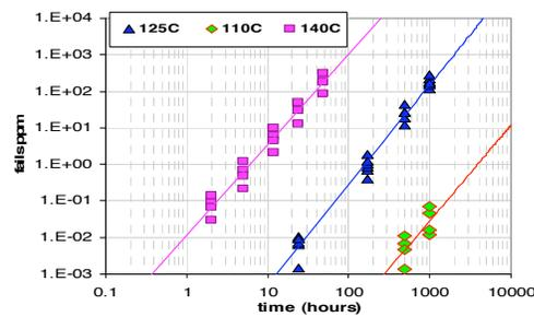
**Fig.4** Data collection for activation energy evaluation. Kinetic of tail bits on 4Mb ePCM macrocell at three different temperatures has been followed.
