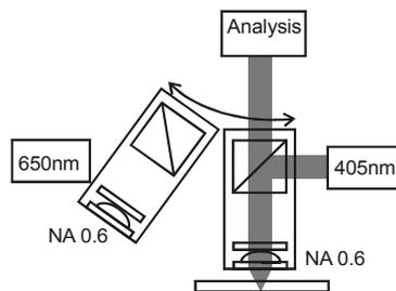
Fig. 1: Schematic of the combined red and blue static tester set up
