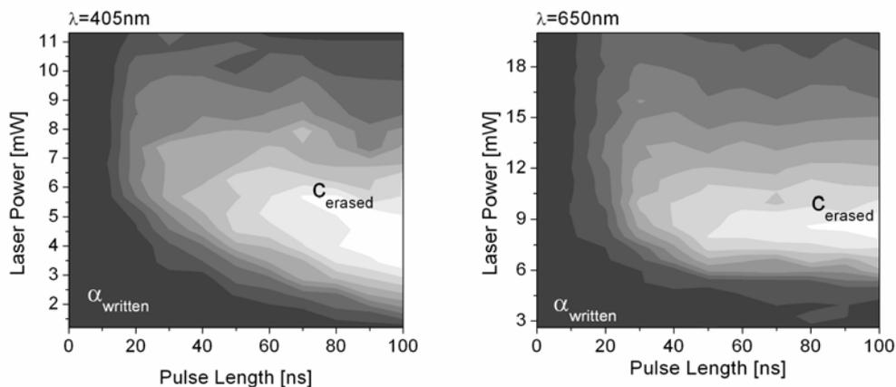
Fig. 2: PTT diagrams of the  $\alpha_{\text{written}}$ - $C_{\text{erased}}$  phase transition of a sample without a nitride interlayer at red (left) and blue (right) laser wavelengths.
