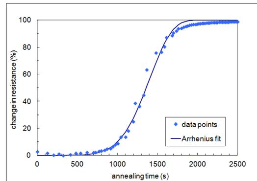
Figure 2: Normalized change in resistivity as a function of annealing time for 132  $^{\circ}\text{C}$ .
