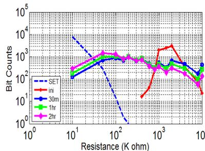
Figure 8: Change in resistance distribution of originally RESET PCRAM cells after baking at 100 °C for Sb-rich Ge-Sb-Te material..
