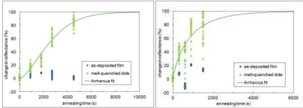
Figure 6: Change in reflectance of as-deposited, amorphous and melt-quenched, amorphous Ge-Sb-Te as a function of annealing time at 90 (left) and 100 °C (right).
