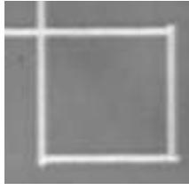
Figure 3: Crystalline box drawn on the amorphous, as-deposited sample by rastering the pump laser over the sample.
