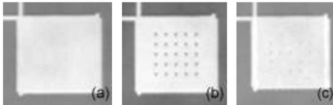
Figure 5: (a) Crystalline square are in as as-deposited, amorphous film. (b) Melt-quenched dots written by a 70 ns pump pulse. (c) Melt-quenched dots partially disappear after heating to  $100^\circ\text{C}$  for 25 min.
