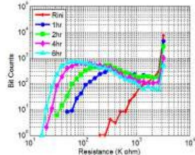
Figure 9: RESET resistance distribution after heating at 190 °C for up to 6h for Ge-rich Ge-Sb-Te material.
