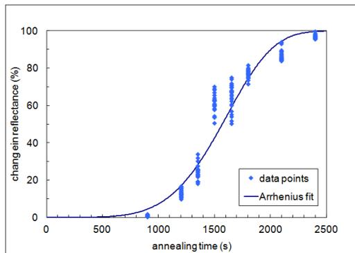
Figure 1: Normalized change in reflectivity as a function of annealing time for 132  $^{\circ}\text{C}$ .
