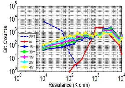
Figure 7: Change in resistance distribution of originally RESET PCRAM cells after baking at 90 °C for Sb-rich Ge-Sb-Te material.
