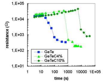
Figure 6: Resistance versus time for GeTe, GeTeC4% and GeTeC10% cells @170°C.
