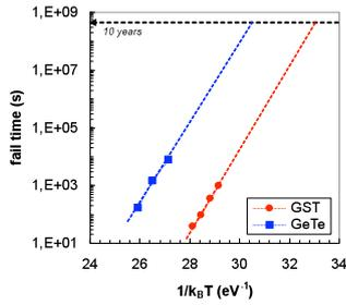
Figure 1: Fail time versus  $1/k_B T$  for GST and GeTe thin films.
