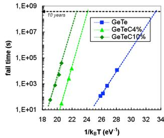
Figure 4: Fail time versus  $1/k_B T$  for GeTe, GeTeC4% and GeTeC10% films.
