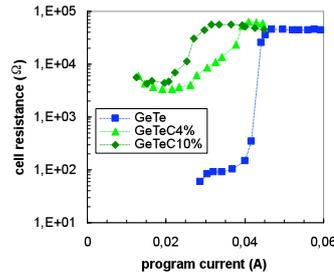
Figure 5: Resistance versus program current for GeTe, GeTeC4% and GeTeC10% memory cells.
