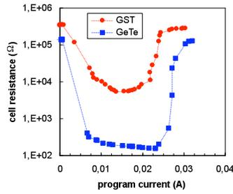
Figure 2: Resistance versus program current for GST and GeTe cells.
