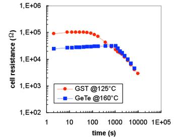
Figure 3: Resistance versus time for GST @125°C and GeTe cells @160°C.
