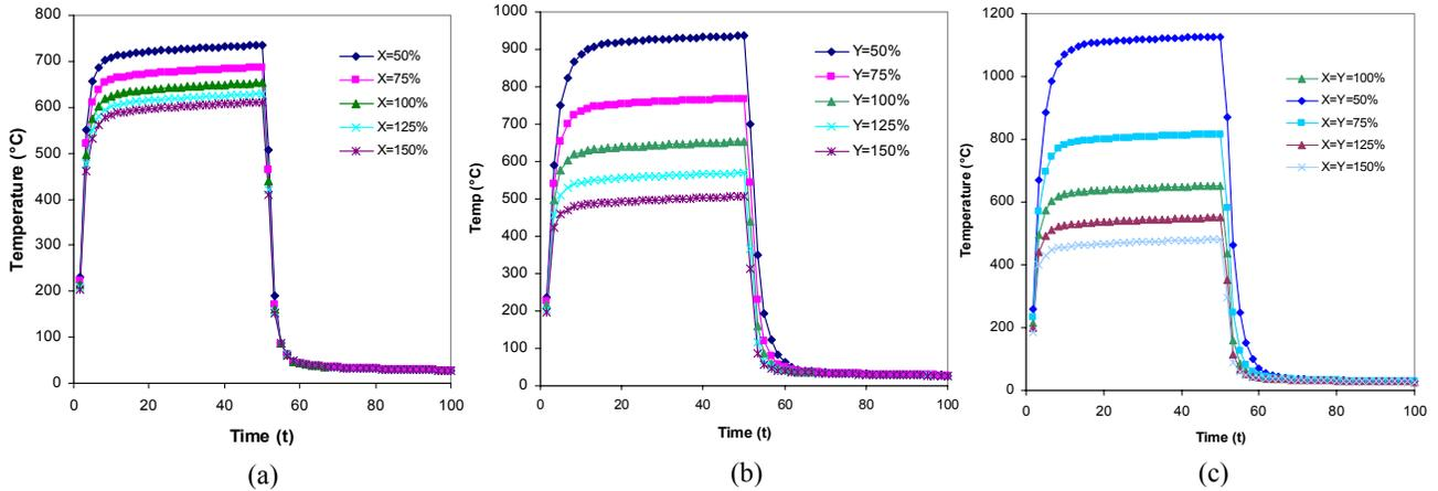
Fig. 5 The temperature history at the phase change layer center with different thermal conductivity (a) in-plane, (b) cross-plane, and (c) both in-plane and cross-plane, respectively for conventional SLL PCRAM.
