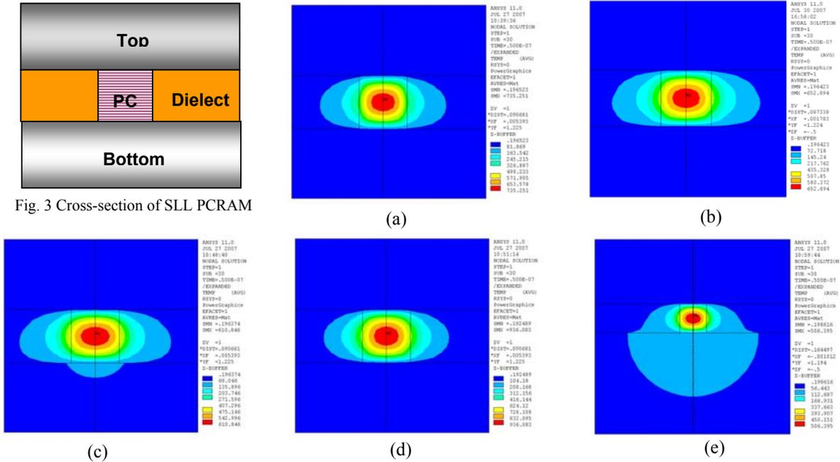
Fig. 4 The cross-sectional views of the temperature distribution in phase change layer with its thermal conductivity of (a)  $X=50\%$ ,  $Y=100\%$ , (b)  $X=100\%$ ,  $Y=100\%$ , (c)  $X=150\%$ ,  $Y=100\%$ , (d)  $X=100\%$ ,  $Y=50\%$  and (e)  $X=100\%$ ,  $Y=150\%$  of that of bulk material, respectively for conventional SLL PCRAM.
