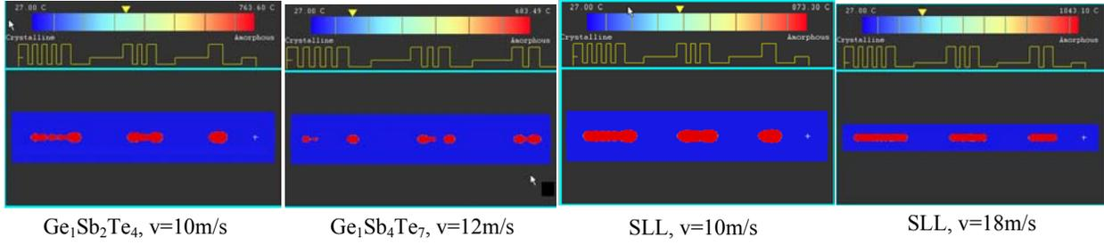
Fig. 1 Mask shapes comparison between discs with SLL structure,  $\text{Ge}_1\text{Sb}_2\text{Te}_4$ ,  $\text{Ge}_1\text{Sb}_4\text{Te}_7$  at different rotation speed
