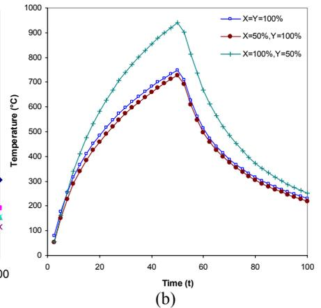
Fig. 9 The temperature history at the PC layer center with (a) isotropical change and (b) anisotropical change of the thermal conductivity for line-type SLL PCRAM.
