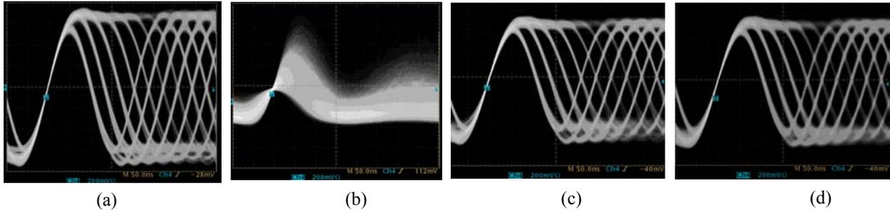
Fig. 2 The eye-patterns of (a)  $\text{Ge}_1\text{Sb}_2\text{Te}_4$  disc 1 $\times$ , 18.9 m/s, (b)  $\text{Ge}_1\text{Sb}_2\text{Te}_4$  disc 10 $\times$ , 18.9 m/s, (c) SLL disc 1 $\times$ , 18.9 m/s, (d) SLL disc 10 $\times$ , 18.9 m/s.
