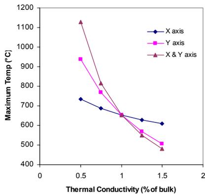
Fig. 6 The maximum temperature achieved for conventional SLL PCRAM with different thermal conductivity.
