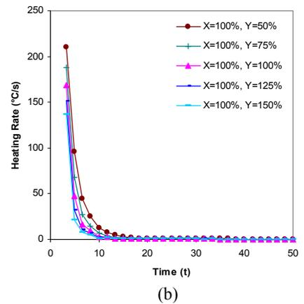
Fig. 7 The heating rate for different thermal conductivity along (a) X-axis, and (b) Y-axis, respectively for conventional SLL PCRAM.
