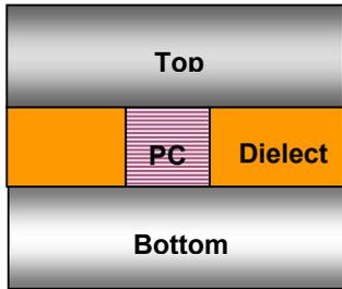
Fig. 3 Cross-section of SLL PCRAM
