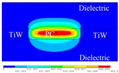
Fig. 8 The cross-sectional view of the temperature distribution in phase change layer with thermal conductivity  $X=50\%$ ,  $Y=50\%$  of that of the bulk for line-type SLL PCRAM.
