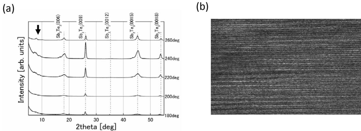
Figure 2 (a) XRD spectra of superlattice films deposited on Si substrates at the temperature from 180 °C to 230 °C (b) TEM image of the superlattice film deposited at 240 °C.
