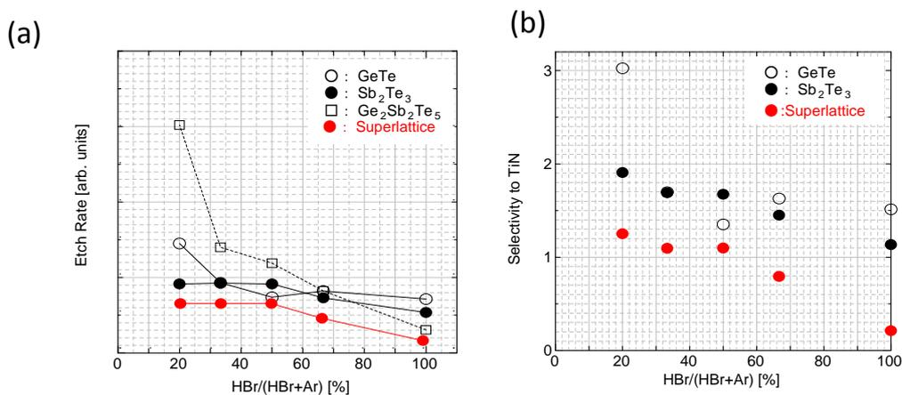
Figure 3 (a) Etching rate of single  $\text{GeTe}$ , single  $\text{Sb}_2\text{Te}_3$ , alloy  $\text{Ge}_2\text{Sb}_2\text{Te}_5$ , and the superlattice (b) Selectivity of the single  $\text{GeTe}$ , single  $\text{Sb}_2\text{Te}_3$ , and the superlattice to the  $\text{TiN}$ .
