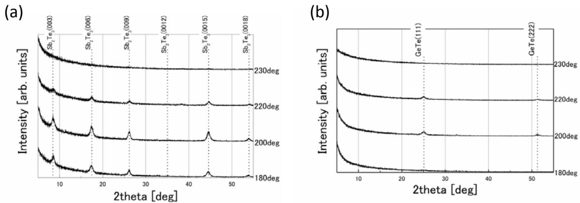
Figure 1 XRD spectra of single  $\text{Sb}_2\text{Te}_3$  (a) and single  $\text{GeTe}$  (b) deposited on Si substrates at the temperature from 180 °C to 230 °C .
