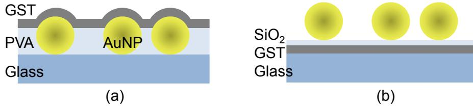
FIG. 1: Schematic of sample structure
