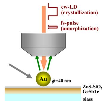
wave (cw) laser diode ( $\lambda=830$  nm) was used to erase the amorphous region by thermal annealing crystallization.
