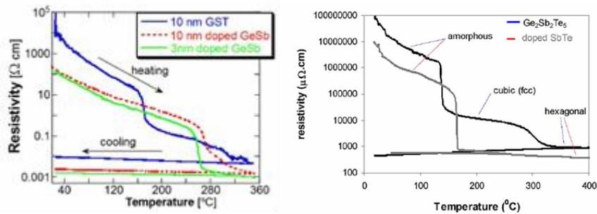
Fig.3: Comparison of the temperature dependent resistivity of as-deposited Ge<sub>2</sub>Sb<sub>2</sub>Te<sub>5</sub> (GST) and doped GeSb film (left side, [20]) and doped-SbTe film (right side, [21]).
