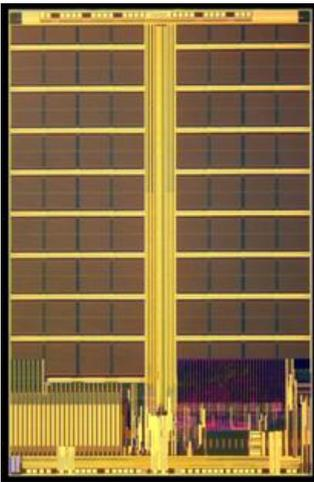
Fig.1: 128Mb Phase Change Memory Device [12, 15].
