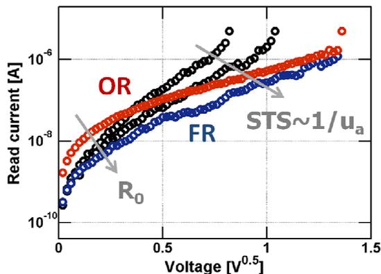
**Fig. 2** Current vs Voltage cell curves for increasing programming pulses. The low-field resistance of the OR state is clearly decreasing while its STS is still increasing
