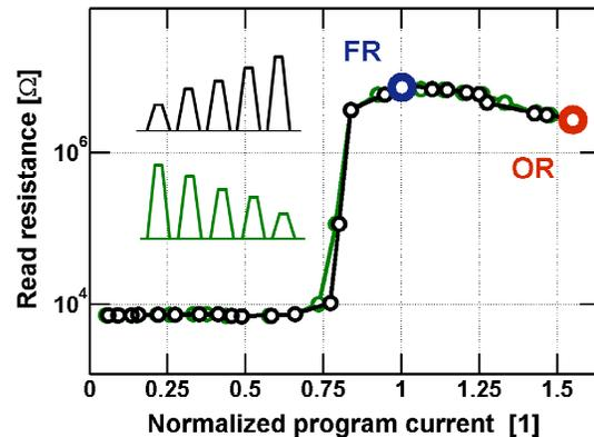
**Fig. 1** Programming characteristics of a PCM for a stair-case up/down pulses (black/green). Full-reset (FR) and Over-reset (OR) are highlighted on both the overlapping curves.
