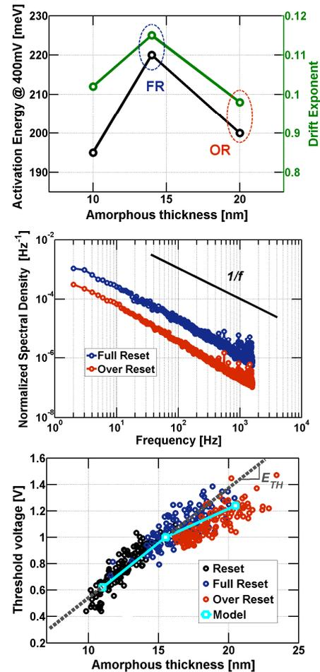
**Fig. 4** From top to down. i) Average (10k cells) activation energy and drift exponent as a function of  $u_a$ . ii) Normalize current noise spectral density: a 3.5x lower noise intensity in the  $1/f$ -like spectra of the OR state is ascribed to both higher  $u_a$  and lower  $E_A$ . iii) Threshold voltage vs extracted amorphous thickness for increasing programming pulses. The switching field saturates in the OR.
