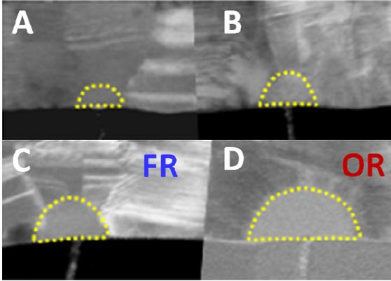
**Fig. 3** TEM images of the amorphized dome for cells programmed with increasing pulses (A through D). OR has a higher and wider amorphous region, according to the electrical extrapolations of  $u_a$  from STS.
