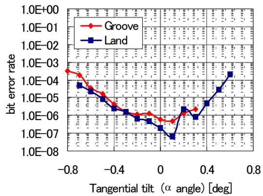
**Fig.4 Bit error rate of 20GB/single-layer disc**
