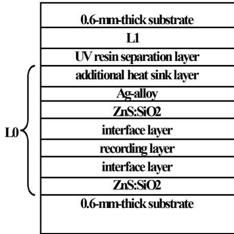
**Fig.6 Cross-sectional View of Dual-layer AOD**
