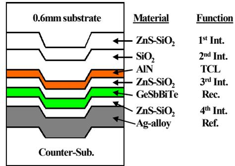
**Fig.1 Cross-sectional View of AOD Medium**
