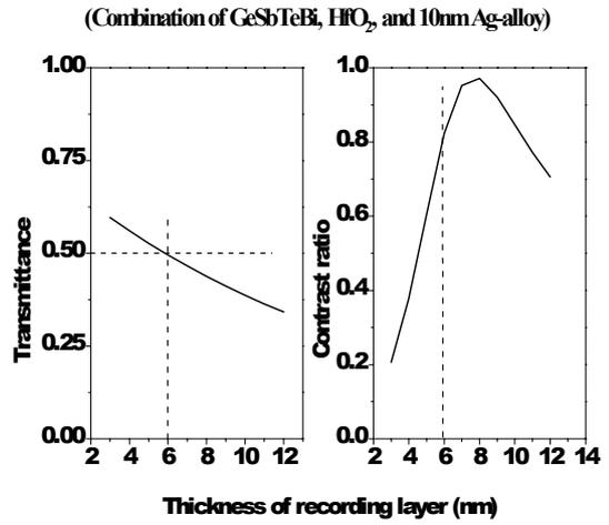
**Fig.7 Example of Optical Design for L0**
