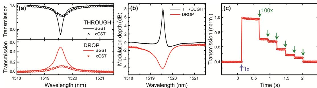
**Fig. 2.** (a) Measured change of the cavity resonance upon switching of the GST. (b) Modulation depth upon crystallization, derived from the data in panel (a). (c) Power coupled to the DROP port of a similar device during one full switching cycle, consisting of one amorphization (blue arrow) and several crystallization (green arrow) steps.
