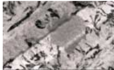
Fig 5(a) – Right - Amorphous mark recorded in crystalline matrix of a fast growth rewritable alloy
