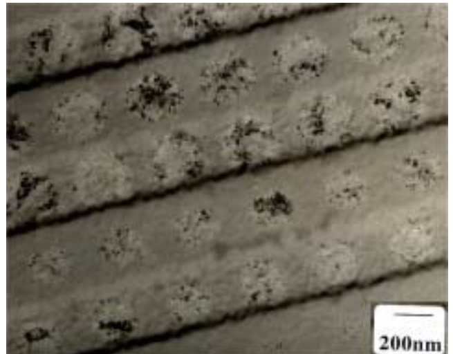
Figure 5(c) UDO Write Once Material. The marks at the top are written at high power, those at the bottom at low power
