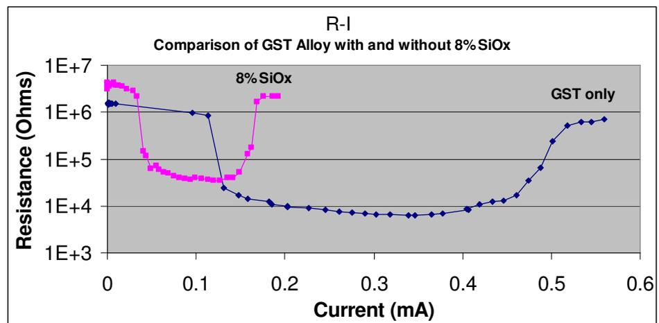
**Figure 15 IVs for 0% and 8% SiOx co-sputtered with GST device on optimized base.**
