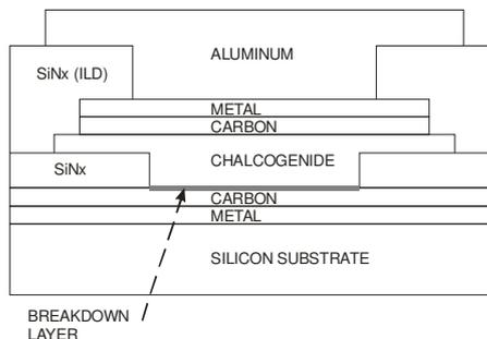
**Figure 1. Schematic of breakdown device**
