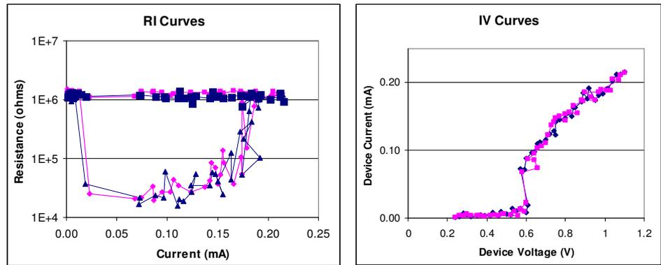
**Figure 5 Current scaling of E-beam devices**
