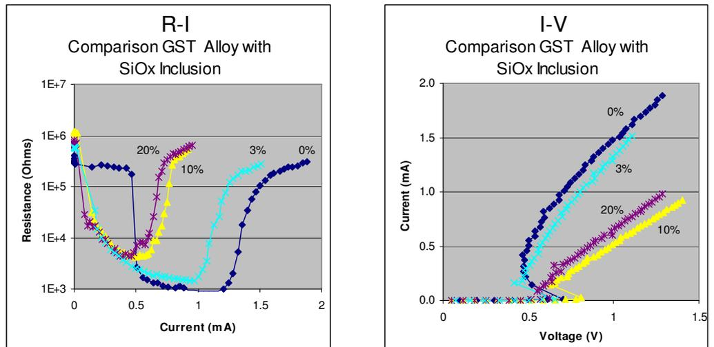
**Figure 13 Programming current reduction for varying co-sputtered percentages with GST.**
