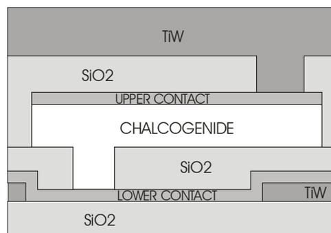
**Figure 2. Schematic of insulated offset pore device**
