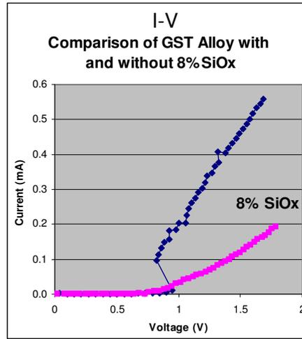
Other composite GST alloys have also been investigated and also show current reduction. Table 1 contains some of these composite alloys, the range investigated and the approximate observed current reduction.
