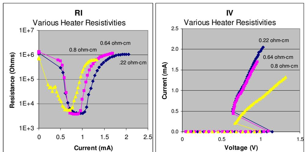
By increasing the resistivity still further, to several milliohm-cm, the current can be further reduced to almost 0.7mA for the smallest 660Å device as shown in Figure 10. Additional, but smaller improvements can be made by minimizing the heat loss through the lower contact still further, as shown in Figure 10 where the resistivity of the metalized layer below the heater is also increased to minimize the heat loss still further and the programming current drops to approximately 0.5mA.
