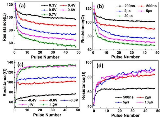
Fig. 2. (a) The gradual resistance tuning under a succession of positive pulses with 5  $\mu\text{s}$  width and different amplitudes, (b) positive pulses with 0.5 V amplitude and different width, (c) negative pulses with 5  $\mu\text{s}$  width and different amplitudes, (d) negative pulses with -1 V amplitude and different width.
