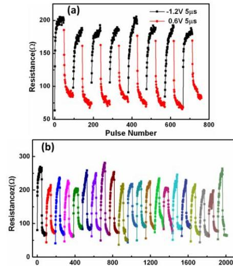
Fig. 3. (a) Repeatability of gradual resistance tuning behavior in Ag/AIST/Ag devices. (b) The gradual resistance tuning behaviors in different cells. Each of the cycles shows the tuning of a cell.
