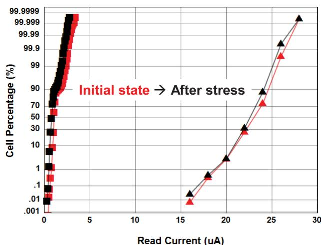
Figure 8. No proximity disturb is seen after stress, which in this case is subjecting the surrounding cells to  $10^6$  programming operations.
