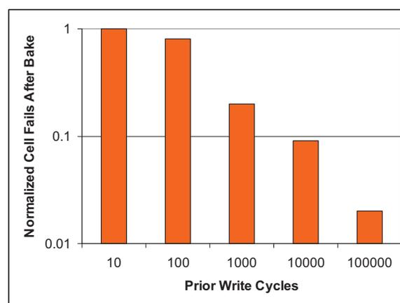
Figure 5. Retention failure rate after an accelerated bake test as a function of prior cycles applied to the array.
