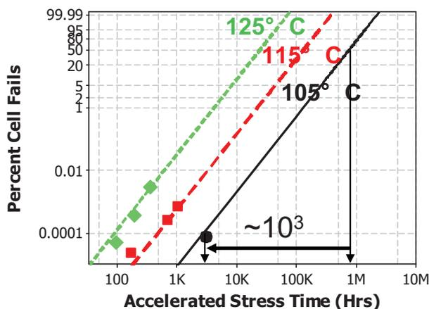
Figure 1. Data from [1] show a 1000x different in failure time between the median (50%) cell and the 1 PPM (0.0001%) cell.
