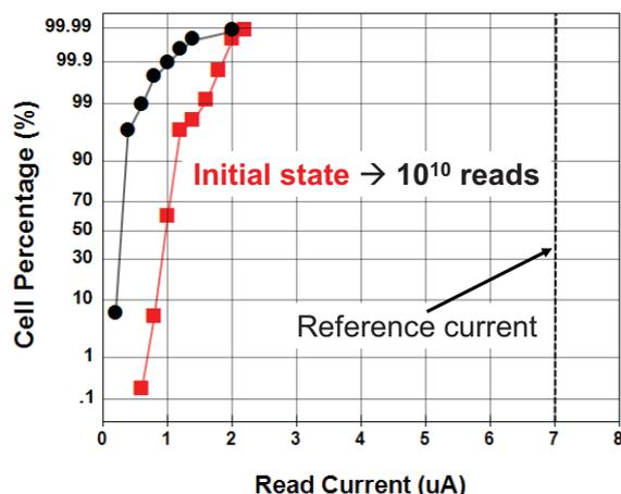
Figure 7. No read disturb (only drift) is observed after  $10^{10}$  reads on reset cells.
