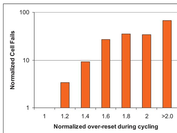
Figure 4. Cell failure rate during cycling as a function of over-reset of the cells.
