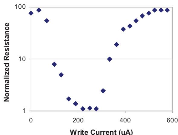
Figure 2. Typical programming curve of a 90nm PCM cell, showing a reset current of  $400 \mu\text{A}$  and a dynamic range of  $\sim 100\times$ .
