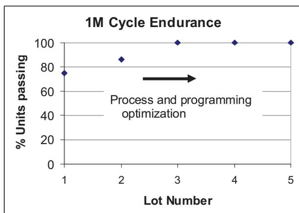
Figure 3. Passing units after  $10^6$  writes, showing the improvement with process and programming optimization.
