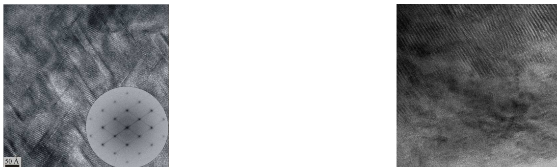
Figure 1: HRTEM image of \text{Ge}_{0.8}\text{Sb}_{0.2}\text{Te} with finite cation defect layers (left, similar structures have been observed for \text{Ge}_{0.25}\text{Bi}_{0.5}\text{Te} ) and of \text{Ge}_{0.25}\text{Bi}_{0.5}\text{Te} (right) showing domains with different arrangements of defect layers and also without defect layers.
