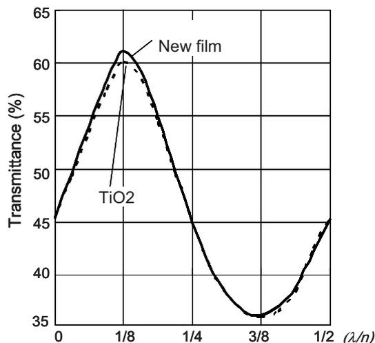
Thickness of the top film with high refractive index
