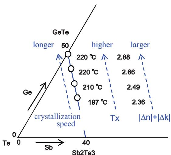
Fig. 2 Compositional dependence of phase-change properties along GeTe-Sb<sub>2</sub>Te<sub>3</sub> tie line
