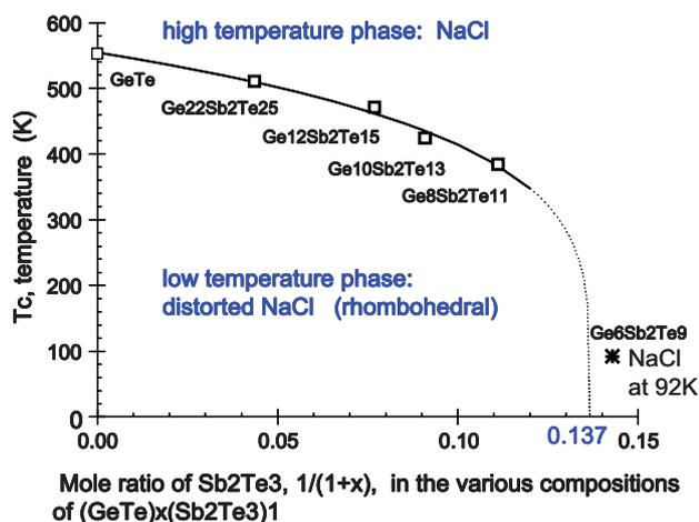
Fig. 3 Compositional dependence of crystal-crystal phase-transition temperature,  $T_c$ , on the increased Sb<sub>2</sub>Te<sub>3</sub> concentration,  $1/(1+x)$ . (the original figure is from the reference[4].)
