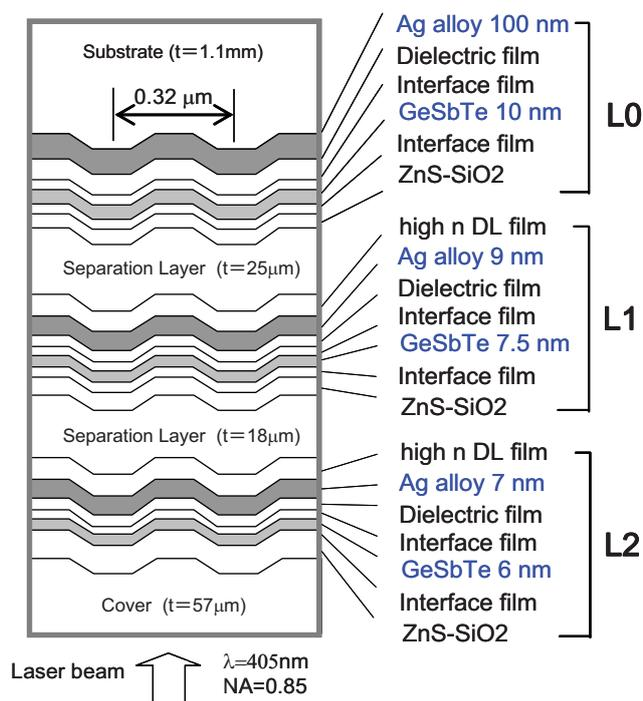
Fig. 1 Cross section of the triple layer optical disk
