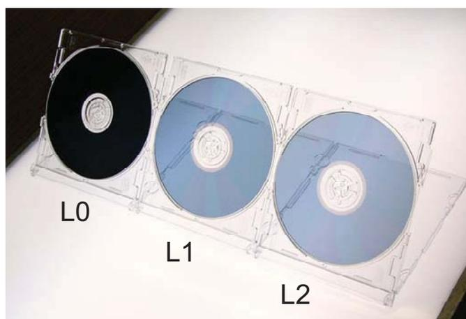
Fig.5 Aspects of L0, and half-transparent L1 and L2 that are made independently for the observation. The triple-layer sample disk was prepared by laminating these three layers.
