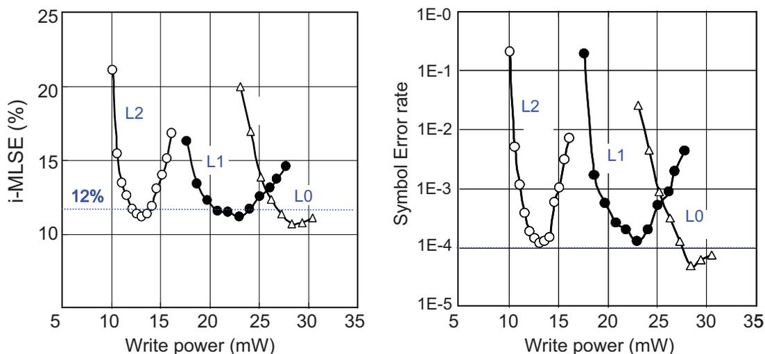
Fig.6 Dependences of i-MLSE (left ) and Sybol Error Rate (right) on write power.
