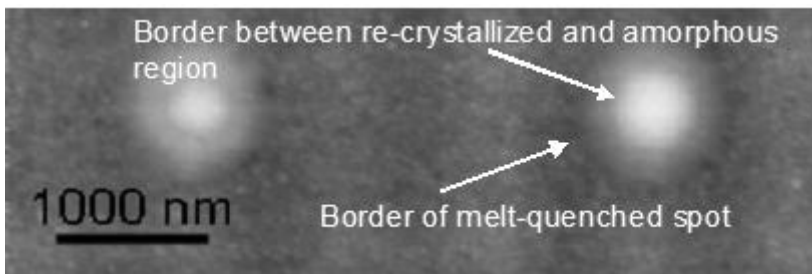
Fig. 9: AFM images of laser spots in crystalline \text{Ge}_3\text{Sb}_6\text{Te}_5 that were first melt-quenched and then attempted to re-crystallize.
