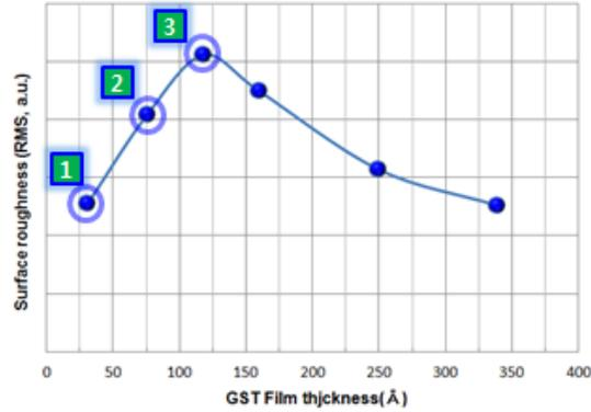
Fig. 2. Surface roughness change of GST films as a function of film thickness.
