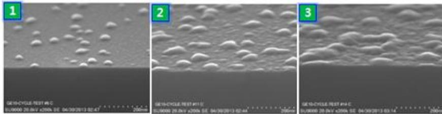
Fig. 3. Surface morphology of GST films with different thickness observed by SEM.
