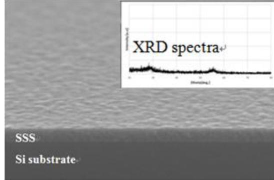
Fig. 8. Surface morphology of as-deposited ALD SSS film (SEM)
