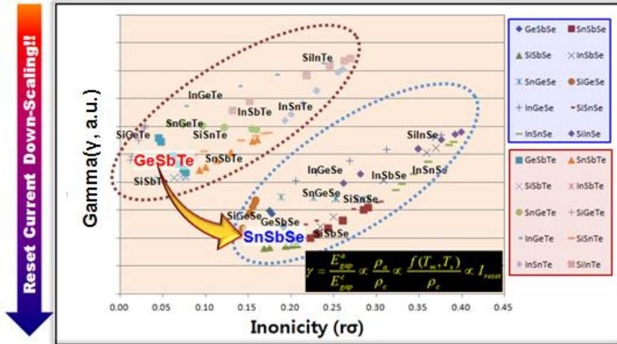
Fig. 5. Resonance bond strength with phase change materials
