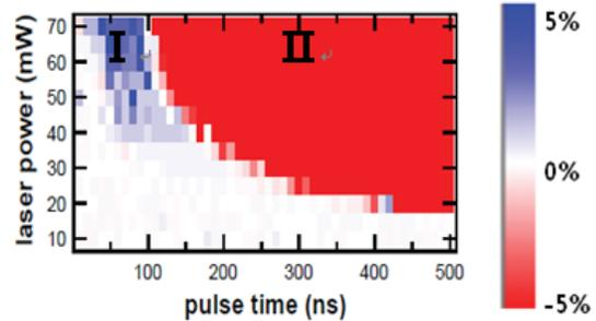
Fig. 10. Contour map of reflectivity variation of as-deposited ALD S-Cube film as a function of laser power and pulse duration.
