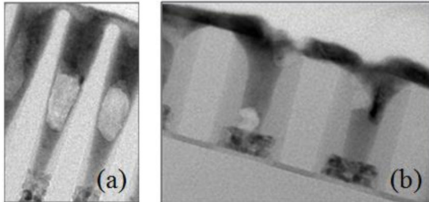
Fig. 1. TEM images of trench holes deposited with GST at each hole size. (a) ~20nm, (b) ~40nm
