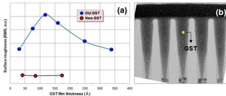
Fig. 4. (a) Change of surface roughness of GST films deposited at different depositions, (b) TEM image of trench hole with new GST.
