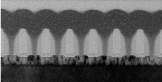
Fig. 9. Gap-filling of ALD S-Cube film using confined cell structure. (Aspect ratio 5.0, Cell dimension of 15nm)
