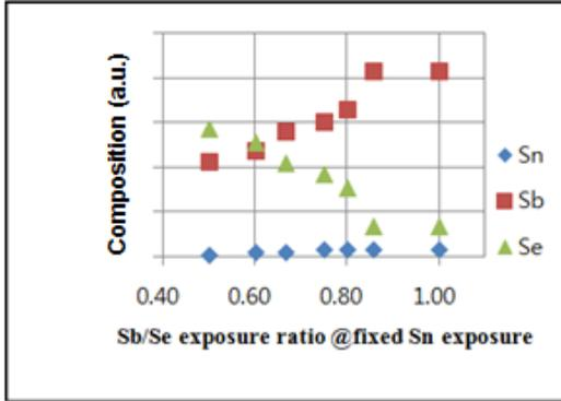
Fig. 7. ALD S-Cube composition with Sb/Se exposure ratio at fixed Sn exposure (Feeding time and sub-cycle)
