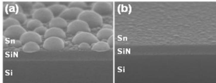
Fig. 6. Growth behavior of ALD single Sn by SEM (a) without in-situ treatment, (b) with in-situ treatment
