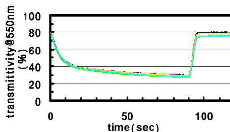
Fig.5 Transmittivity dependence on time. Applied voltage is +1.5 V (colored) and -1.5 V (bleached).
