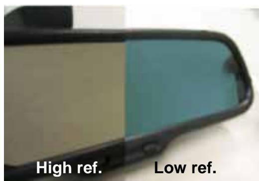
Fig.3 Glare-free inner mirror using  $WO_3$  electrochromic cell
