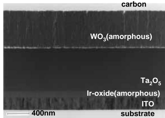
**Fig.6 Cross-sectional TEM image of a transparent  $\text{WO}_3$  electrochromic cell**
