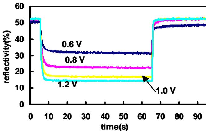
**Fig.7 Transient characteristic and bias voltage dependence of electrochromism in reflective electrochromic cell**
