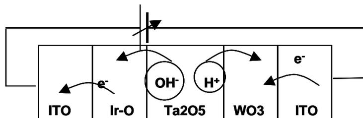
Fig.2 Example of electrochromic cell
