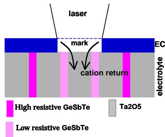
Fig.10 Solid electrolyte composed of  $Ta_2O_5$  and GeSbTe
