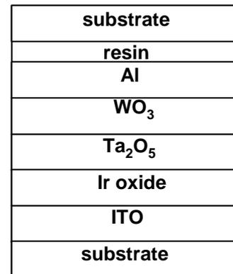
**Fig.8 Schematic layer structure of reflective electrochromic cell**
