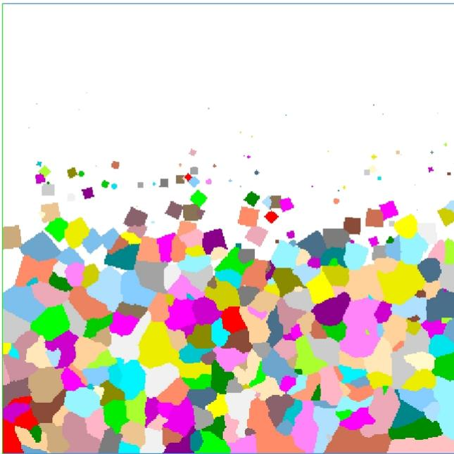
Fig. 1. A two-dimensional CA-FE microstructural simulation showing the grain structure in an Al - 3.5wt.% Mg alloy during solidification at  $\sim 10^{-3} \text{ m s}^{-1}$  in a temperature gradient of  $10^4 \text{ K m}^{-1}$ . The area shown represents  $1 \text{ mm}^2$ . The temperature decreases from top to bottom, and the featureless area at the top is the liquid ahead of the solidification front. (courtesy T. E. Quested)
