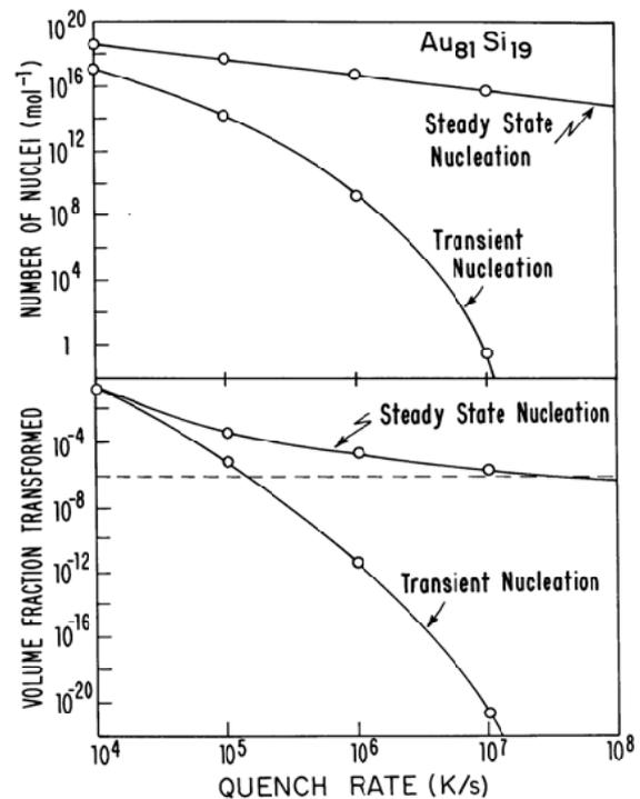
Fig. 2. The number of nuclei (a) and transformed volume fraction (b) calculated for quenching the marginal metallic glass-forming alloy Au<sub>81</sub>Si<sub>19</sub> (at.%) from the equilibrium liquid state at various rates, assuming steady state or transient nucleation. (from [16])
