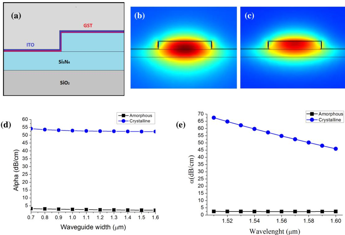
**Fig. 1:** (a) Waveguide geometry and materials used in the FEM simulation. (b) Calculated TE<sub>0</sub> modal profile when the GST is in the amorphous state and (c) when it is in the crystalline state. (d) Absorption coefficient against width of the waveguide for a wavelength of  $\lambda=1.57 \mu\text{m}$ . (e) Absorption coefficient dependence on the wavelength for a width of  $1.3 \mu\text{m}$ .
