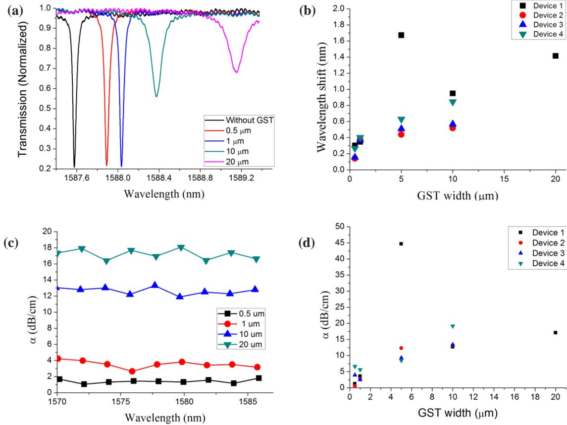
**Fig. 4:** (a) Transmission spectrum of devices 1 with their respective resonance peaks for different GST width. (b) Average of the wavelength shift due to the GST coverage for every device. (c) Absorption coefficient as a function of the wavelength for the devices 1 and (d) Absorption coefficient as a function of the GST width for every device.
