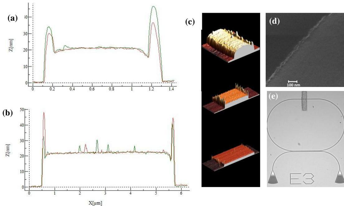
**Fig. 3:** AFM profile for the GST layers with width of (a) 0.5  $\mu\text{m}$  and (b) 5  $\mu\text{m}$ . (c) From top to bottom: 3D AFM images for GST widths of 0.5, 5, and 20  $\mu\text{m}$ . (d) SEM image: border of the 5  $\mu\text{m}$  GST layer. (e) Device with GST on top at the end of all the fabrication process.
