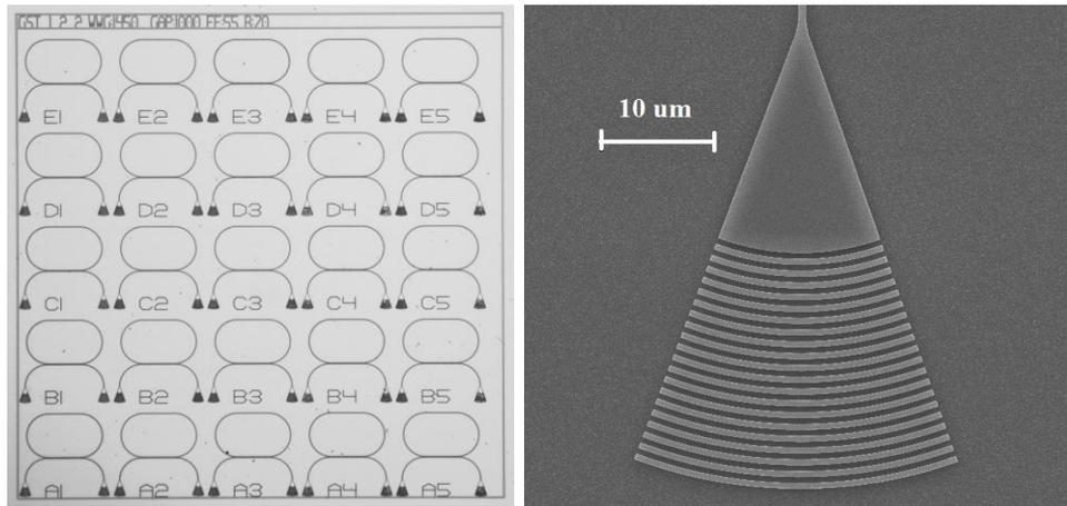
**Fig. 2:** *Left:* Optical micrograph of half-etched  $\text{Si}_3\text{N}_4$  waveguides and microring resonators. The grating couplers were designed for five different wavelengths in the range  $1.5\text{-}1.6\ \mu\text{m}$  and for five different (after) GST widths. *Right:* SEM image of a grating coupler designed for a wavelength of  $1.52\ \mu\text{m}$
