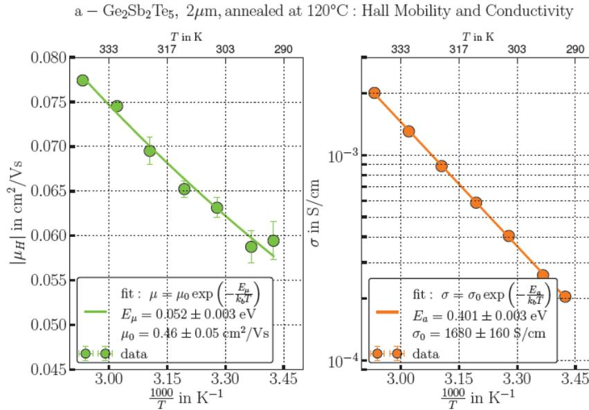
**Figure 2:** Hall mobility (left) and conductivity measurements (right) of an amorphous as-deposited  $\text{Ge}_2\text{Sb}_2\text{Te}_5$  sample taken in a temperature range from 290 – 340 K. The Hall mobility increases weakly with temperature, whereas the conductivity increases by an order of magnitude. These increases correspond to activation energies of  $E_\mu = 0.05$  eV and  $E_a = 0.4$  eV, respectively.
