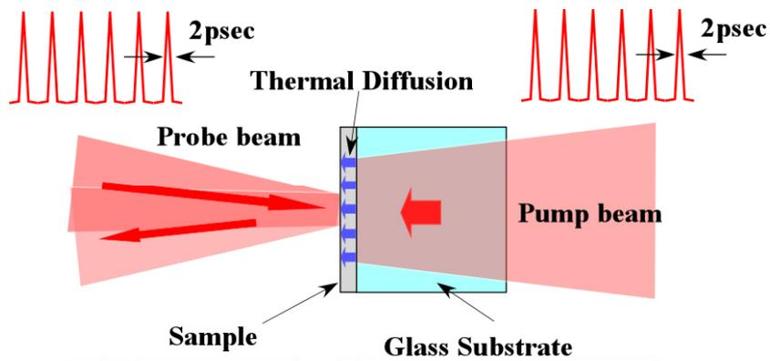
**Figure 3.** Schematic sketch of the thermo-reflectance measurement.
