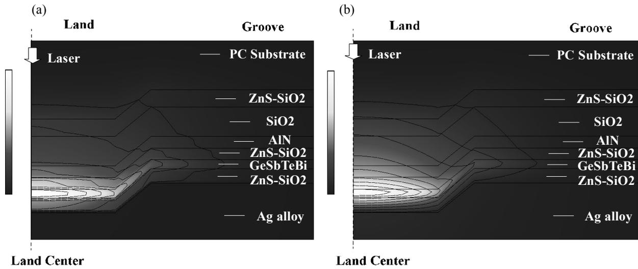
**Figure 8.** Temperature distribution in the medium. (a) considering  $R_B$ , (b) without considering  $R_B$ .
