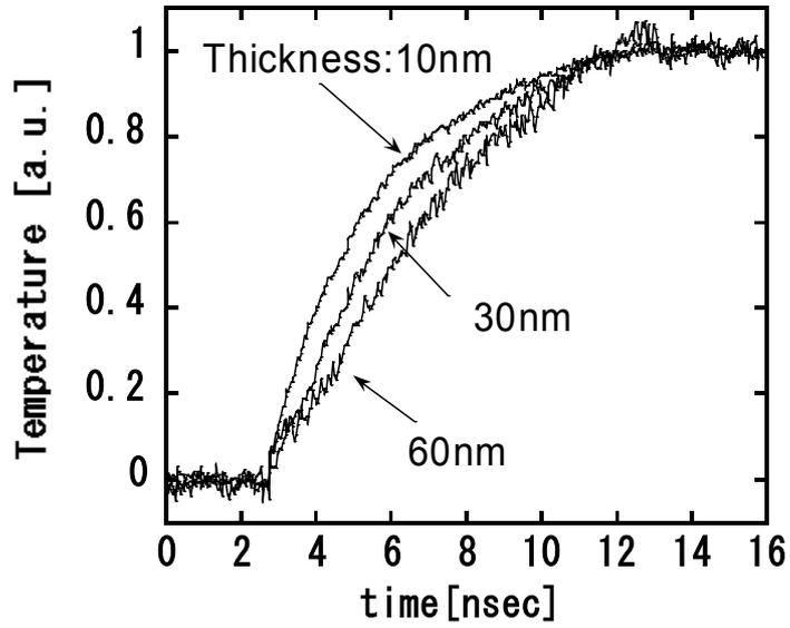
**Figure 5-(a).** Temperature history curves of three-layer samples of Mo/GeSbTeBi/Mo thin films for three different GeSbTeBi film thicknesses.
