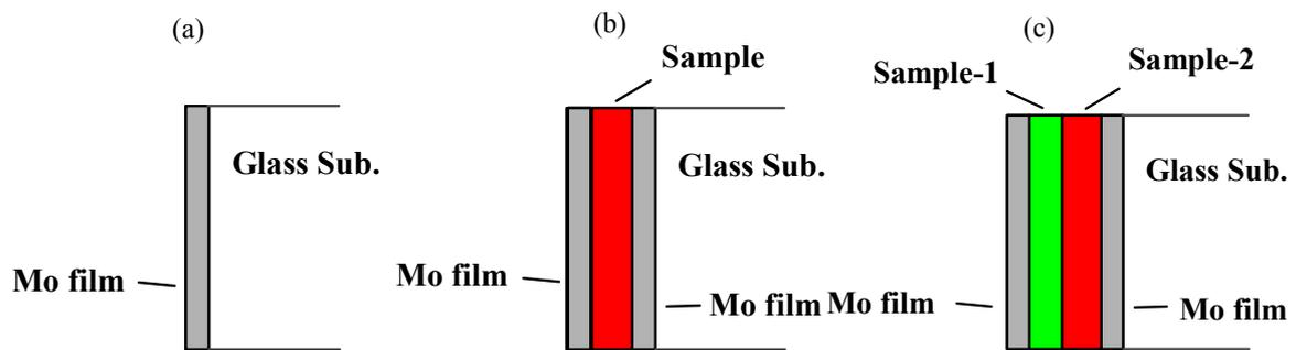
**Figure 4.** Sample structures for the thermo-reflectance measurement. (a) single-layer Mo, (b) a ZS or GSTB film sandwiched by two Mo films, and (c) Mo/ZS/GSTB/Mo films.
