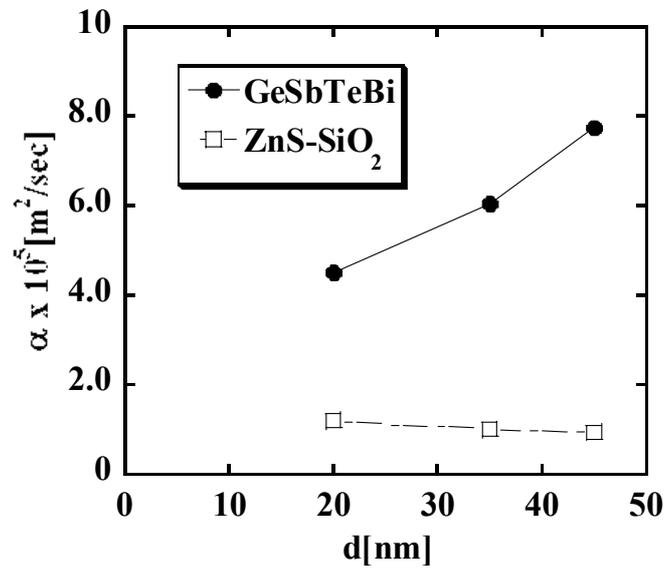
Figure 6. Thermal diffusivity of GeSbTeBi and ZnS-SiO<sub>2</sub> films as a function of film thickness.
