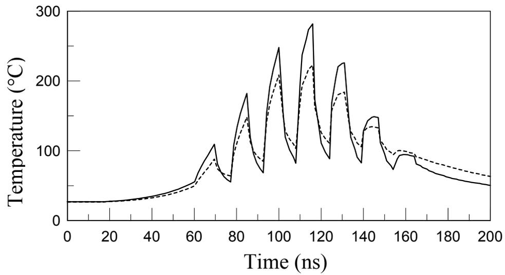
**Figure 9.** Temperature evolution during multi-pulse application on the neighboring track. Solid line:  $R_B$  considered, dotted line: without  $R_B$ .
