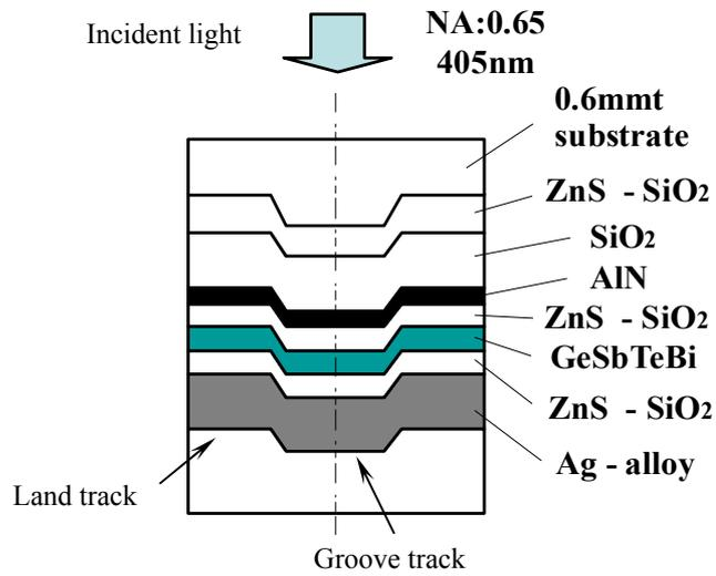
**Figure 1.** Film structure of rewritable HD DVD medium (HD DVD-ARW) used in this study.
