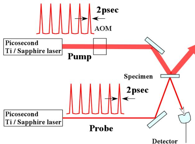
**Figure 2.** Block diagram of the pico-second thermo-reflectance measurement system. AOM stands for acoustic optic modulator.
