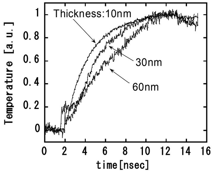
**Figure 5-(b).** Temperature history curves of three-layer samples of Mo/ZnS-SiO<sub>2</sub>/Mo thin films.
