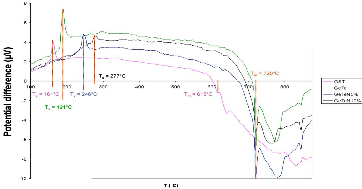
*Figure 1:* Differential Thermal Analyses of GST, GeTe and two nitrogen-doped GeTe. The crystallization temperatures and melting temperatures are reported on the graph.
