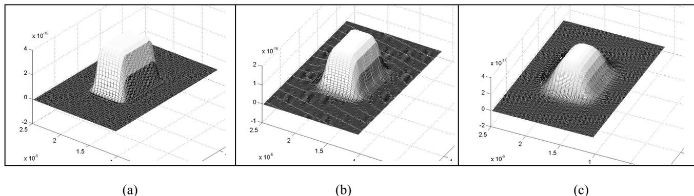
Fig. 4. Simulated EFM images of a 300x500nm 'bit' written into a phase-change medium for tip-sample separations of (a) 20nm, (b) 60nm and (c) 120nm. Scanned area is 1.5x0.9 $\mu$ m.
