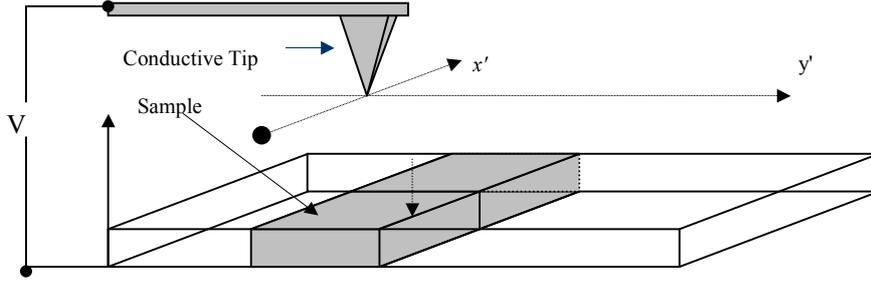
**Fig. 1** General tip-sample arrangement for electric force microscopy
