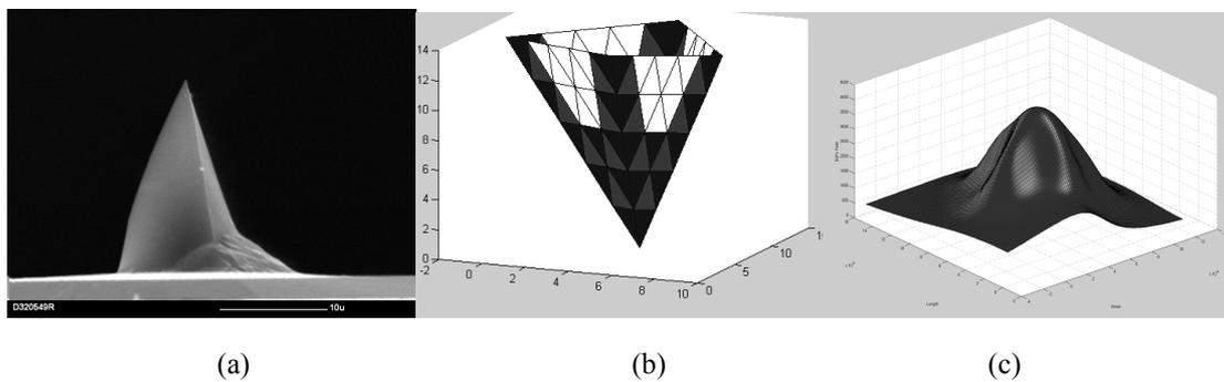
Fig. 2. (a) SEM image of typical AFM tip, (b) distribution of triangular charge sheets on tip surface, (c) electric field distribution below tip with charge distribution of (b)
