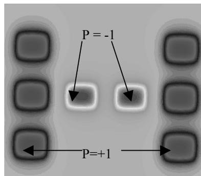
Fig. 3. EFM image of 300x500 nm rectangular bits or domains in a ferroelectric material with a normalized polarization  $\pm 1$  and for a tip-sample distance is 60 nm.
