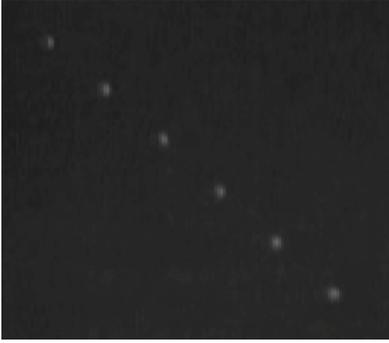
Figure 1. CCD image of amorphization marks with both single pulse and multi-pulse excitation. (from top left to bottom right, a single pulse of 18.7 mJ/cm<sup>2</sup>, 4 pulses of 17.4 mJ/cm<sup>2</sup>, 24 pulses of 16.2 mJ/cm<sup>2</sup>, 230 pulses of 14.9 mJ/cm<sup>2</sup>, 2300 pulses of 13.9 mJ/cm<sup>2</sup>, 51120 pulses of 12.5 mJ/cm<sup>2</sup>)
