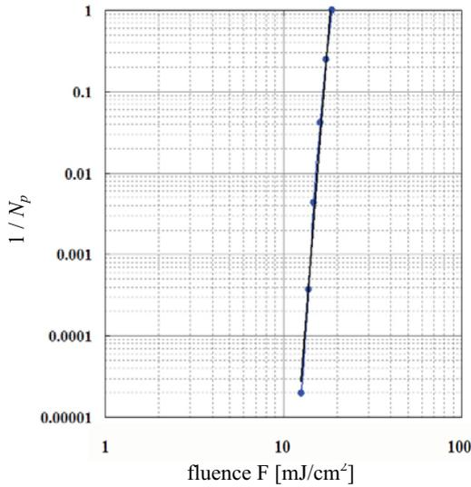
Figure 4. Relation between the excitation intensity and the amorphized volume fraction per pulse which is proportional to  $1/N_p$ .
