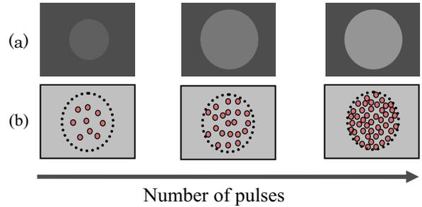
Figure 3. (a) (from left to right) Demonstration of amorphous mark contrast enhancement while increasing the number of excitation pulses.(b) Corresponding illustration of Ge switching area increment as the number of excitation pulses increase.
