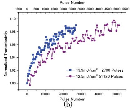
Figure 2. Transmission efficiency as a function of pulse number for difference fluencies (a) fluencies = 17.4, 16.2 and 15.1 mJ/cm<sup>2</sup>. The above horizontal axis corresponds to the red and orange curves, while the bottom horizontal axis corresponds to the green curve. (b) fluencies =13.9 and 12.5 mJ/cm<sup>2</sup>. The above horizontal axis corresponds to the blue curve while the bottom horizontal axis corresponds to the purple curve.
