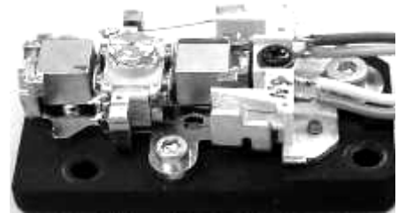
Fig. 2. A picture of 2-axis actuator for NFR. SIL of NA 1.84 is assembled.
