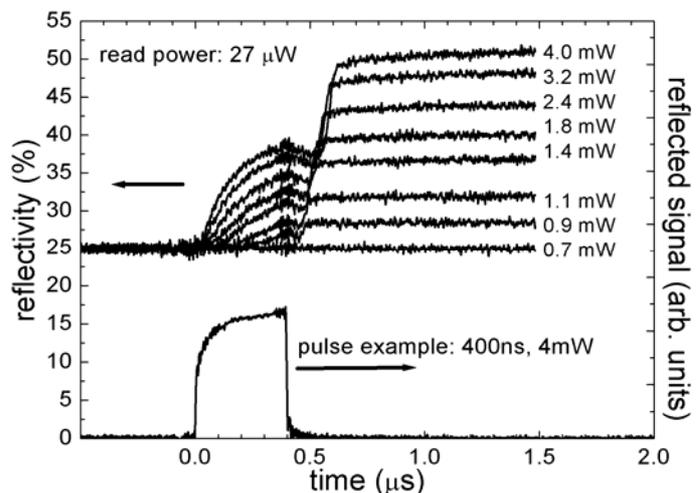
**Fig.2.** Reflectivity versus time as measured before, during, and after a  $\tau_w = 0.4\ \mu\text{s}$  pulse of varying power  $P_w$ . From top to bottom, the traces correspond to  $P_w = 4.0, 3.2, 2.4, 1.8, 1.4, 1.1, 0.9,$  and  $0.7\ \text{mW}$ , respectively. The CW read power is fixed at  $P_R = 27\ \mu\text{W}$ .
