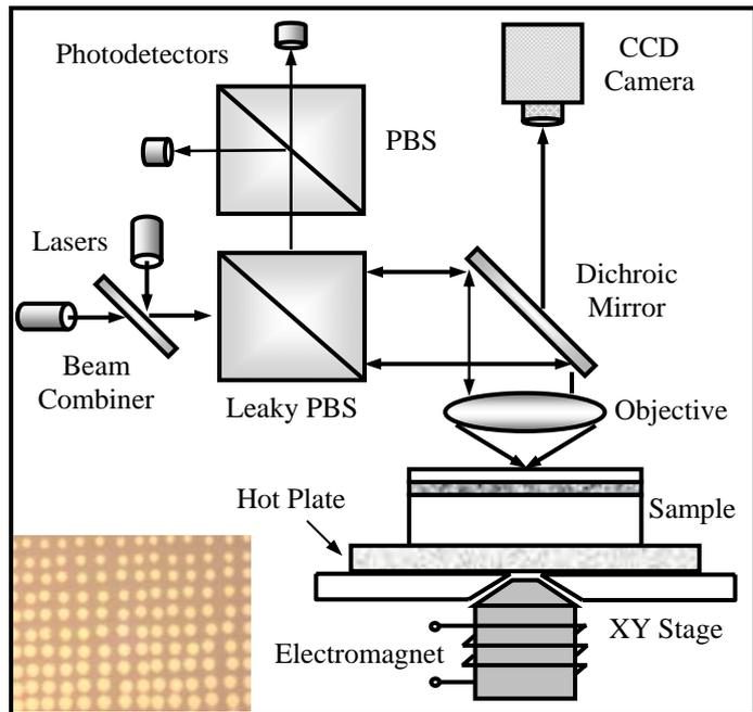
**Fig.1.** Diagram of the measurement system. Beams from two lasers of differing wavelengths are combined and focused on the active layer of the sample; reflected beams are monitored in real time by fast photodiodes. The sample stage can be translated in small steps.
