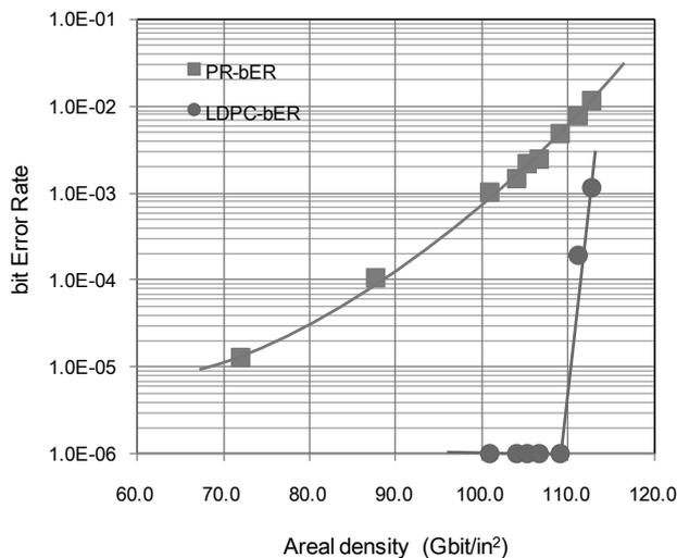
Fig. 3. Dependence of the bit error rate on the areal recording density.
