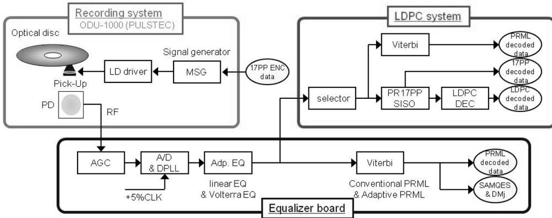
Fig. 1. Block diagram of the recording system, equalizer board and LDPC board.
