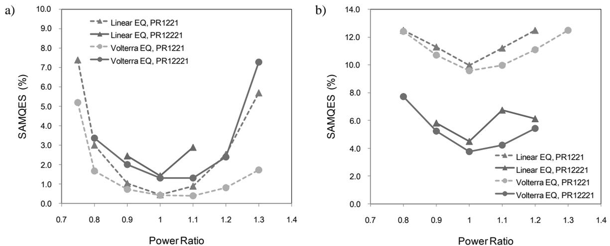
Fig. 2. The recording power dependence of SAMQES values on three consecutive tracks. (a)  $72.0 \text{ Gbit/in}^2$  (b)  $100.8 \text{ Gbit/in}^2$ .
