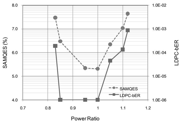
Fig. 4. Recording power tolerance of a phase-change disc at an areal density of 109 Gbit/in<sup>2</sup>.
