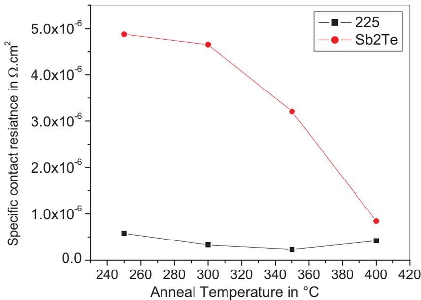
Figure 2: Change the extracted specific contact resistance measured for 225 and doped-Sb<sub>2</sub>Te to TiW with annealing temperatures from 250°C to 400°C.
