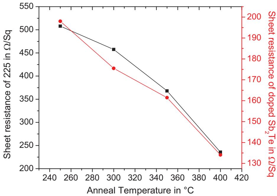
Figure 1: Change in the sheet resistance measured for 225 and doped-Sb<sub>2</sub>Te at room temperature with annealing temperatures from 250°C to 400°C.
